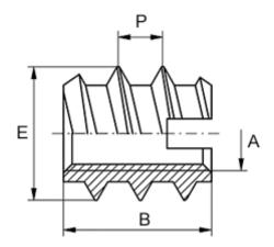
Female thread A = M10Length B = 23Male thread E = 16.0Min hole depth = 26
